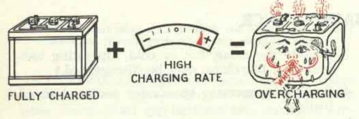
(2) Fully Charged Battery and a High Charging Rate—This usually indicates that the voltage regulator unit either is not limiting the generator voltage as it should or is set too high. A high charging rate to a fully charged battery will damage the battery and the accompanying high voltage is very injurious to all electrical units.
