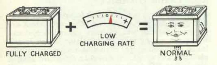
Fully Charged Battery and Low Charging Rate—This indicates normal generator-regulator operation.
