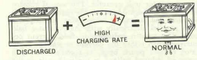
(3) Low Battery and High Charging Rate—This is normal generator-regulator action. Regulator setting may be checked as outlined in the following section.
